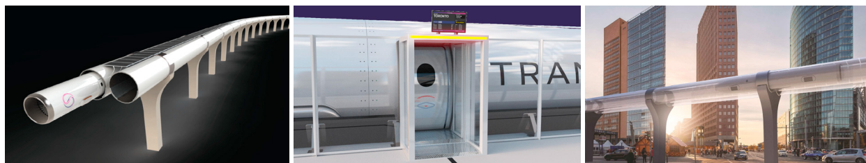
Fig. 1. TransPod system: The M2A vehicle resembles an aircraft fuselage, using electromagnetic propulsion, moving in a steel tube guideway which is twinned for bidirectional vehicle flow (left: front of vehicle; middle: open station guideway; right: image shows transparency for clarity).
